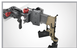
Position the lower receiver to install pivot pin, spring & detent. ( Smart-Fit sold separately )
