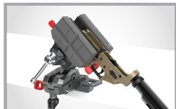
Optimally position lower receiver to install buffer and buffer detent pin.
