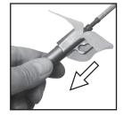
STEP 4: Re-attach the slotted bore patch tip or bore patch jag to the rod (along with a clean patch). Push the clean/dry patch through the bore from action to muzzle. The patch will absorb loosened fouling. Repeat steps 2 through 4 using multiple patches until last patch comes out clean.
