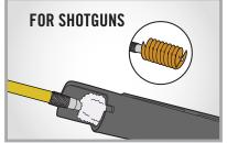
Use brush and mop to loosen and remove fouling from shotgun bore
