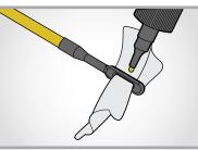
Use slotted patch tip to apply solvent to bore
