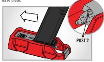
**Step 2:** Place magazine on top of tool and insert post 2 into base plate port. **Step 3:** While pressing down, slide the magazine backrward to remove the base plate and capture the spring.
