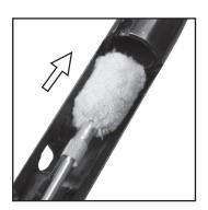
**STEP 5:** Once the bore is clean, wipe down the action with a clean patch, lightly coated in gun solvent, to remove any stray fouling. Finally, wipe down action with clean/dry patch to remove any excess solvent.
