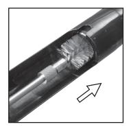
**STEP 4:** Attach the correct size bore mop to the rod. Push the mop through the bore from action to muzzle. The mop fibers will push-out loose fouling. Repeat steps 2 through 4 until clean.
