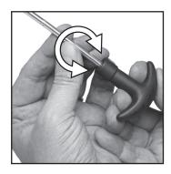
STEP 2: Attach the slotted bore patch tip to the adapter end of the assembled rod. Slide a cleaning patch through the slotted tip. Apply a generous amount of gun solvent to the patch and push the patch through bore. This step moistens and begins to loosen fouling.
