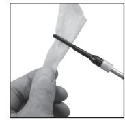
**STEP 3:** Remove the slotted bore patch tip from the rod and attach the appropriate size bore brush to the rod. Push the bore brush through the bore from action to muzzle. This step loosens more fouling.
