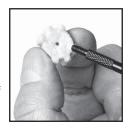
STEP 4: Locate the rotating threaded section on the rod handle. Using the rotating threads, connect the appropriate number of rods to clean the full length of the rifle's bore.
