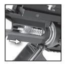
**STEP 3:** Replace the chamber brush with the male thread adaptor and a wool star chamber pad. Apply a few drops of solvent to star chamber pad. Insert star chamber pad and rotate clockwise to absorb the loosened fouling. Repeat this step using additional star chamber pads until they come out clean.
