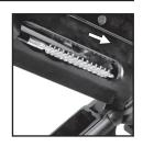
STEP 8: Re-attach the slotted tip to the rod, then push a clean patch through the bore. This patch will absorb loosened fouling. Repeat steps 5 through 8 until the last patch comes out clean.
