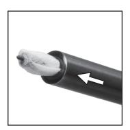
**STEP 2B - JAGS:** Pierce the center of an appropriately sized cleaning patch with the tip of the jag and wrap the patch around the jag. Apply a generous amount of gun solvent
