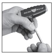
**STEP 3:** Remove the slotted tip or jag from the rod and attach the appropriate size brush to the rod. Push the brush through the bore from action to muzzle. This step loosens more fouling.
