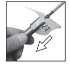
**STEP 5:** Once the bore is clean, wipe down the action and its parts with a clean patch lightly coated in gun solvent to remove any stray fouling. Finally, wipe down action with a clean dry patch to remove any excess solvent.
