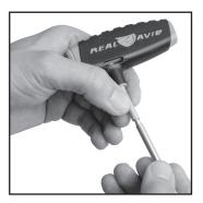
**STEP 3:** Remove the slotted bore patch tip or jag from the rod and attach the appropriate size brush to the rod. Push the brush through the bore from action to muzzle. This step loosens more fouling.
