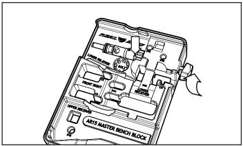
**BOLT EJECTOR:** The bolt ejector is retained by a 1/16" roll pin. The roll pin is under tension from the spring loaded ejector. To relieve the tension, lay the bolt onto the bench block as shown and tighten the bolt ejector compression screw, then remove or install the roll pin.
