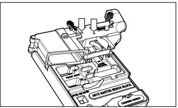
**TRIGGER ASSEMBLY:** The trigger assembly can be removed by knocking out two 5/32" pins located on the side of the lower receiver. Lay the lower receiver on its right side as shown and use a 5/32" punch to remove these two pins. **Note that the pistol grip should be removed for proper fit.**
