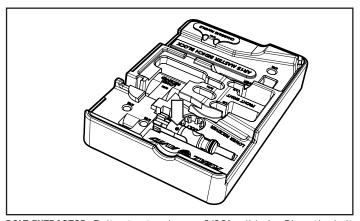
**BOLT EXTRACTOR:** Bolt extractors have a 3/32" solid pin. Place the bolt on its side as shown and tap out pin with a 3/32" punch.
