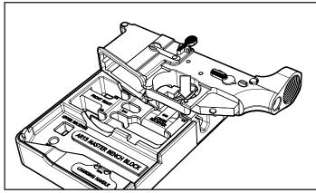
**TRIGGER GUARD:** The trigger guard can be removed from many lower receivers. For proper removal, lay the lower receiver on its right side as shown and use a 1/8" punch to remove the trigger guard pin. **Note that the pistol grip should be removed for proper fit.**
