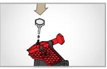
**Step 2**. Load spring first, then detent second into the PPT fixture. Compress the spring and detent with the PPT plunger and hold.
