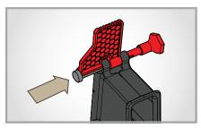
**Step 4.** Insert pivot pin as shown, then remove large PPT pin. Finally, remove PPT fixture and snap pivot pin into closed position.
