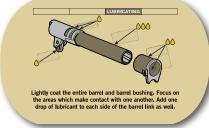
Critical lubrication points are highlighted and explained
